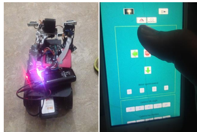
Fig. 8 Direction controlling of emr through the web.
