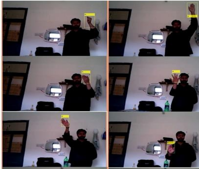
Figure 6 Hand detected by combination cascade detector and skin detector
